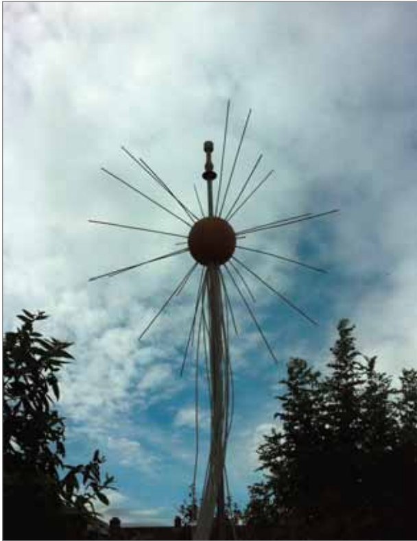
Figure 9: Prototype three-dimensional anemometer, called a Metometer, in author's back yard
