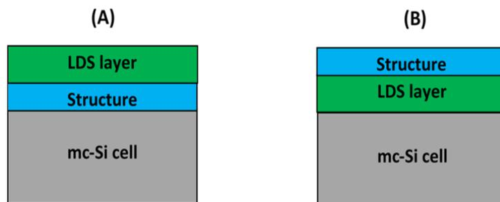
**Figure 2:** Initial designs for a structure-enhanced luminescent down-shifting (SE-LDS) mc-Si device with the selectively reflecting 'Bragg' structure situated (A) below the LDS layer and (B) above the LDS layer
