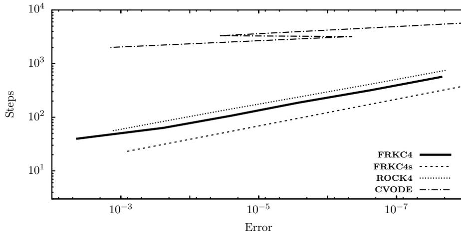
Figure 6: Performance results derived from the estimated error for the Brusselator problem. Shown are data for the fourth-order ESRK schemes **FRKC4s**, **FRKC6s**, **ROCK4**, and the fifth-order implicit **CVODE** scheme.
