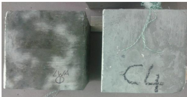
Fig. 2. Leakage of PCM from the lightweight aggregate carrier
