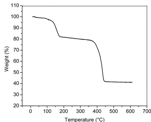
**Fig. 3** TGA plot of the xerogel (80 °C).
