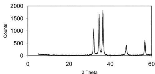
Fig. 1 X-ray powder diffraction plot of ZnO material calcined at 500 °C.
