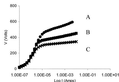
**Fig. 7** I–V curve of varistor samples sintered at 1050 °C/2 hr. A = varistors prepared from “core shell” samples. B = varistors prepared from nano-ZnO and metal oxides C = commercial varistor (the average thickness of the pellets was 0.65 mm).
