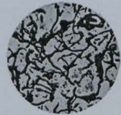
Micro-photograph of Ordinary Cast Iron
