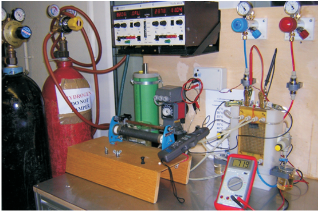
Figure 8. Operational Single Cell Test Bed.
