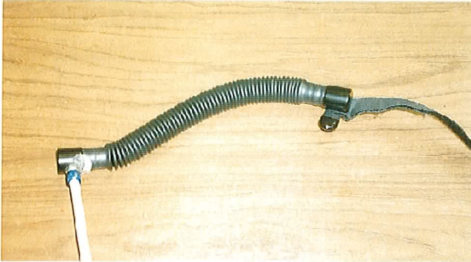
Figure 3.2: Pressure Coil used in the Initial Prototype.
