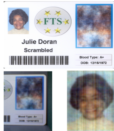
Fig. 6. Example of a security card designed to include a texture code of the holders portrate (top). The images (i.e. portrate and texture code) have been printed onto the identity card at 600dpi. An image of this card (bottom-left) has been generated using a mobile phone. After cropping the texture code obtained from this low resolution data, a reconstruction can still be obtained as shown (bottom-right).
