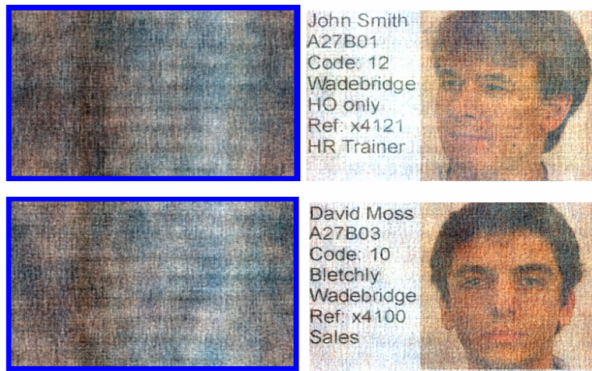
Fig. 7. Example of the diffusion of composite images with the inclusion of a reference frame for enhancing and automating the processes of cropping and orientation. In each case the data fields have been printed and scanned at 300 dpi.
