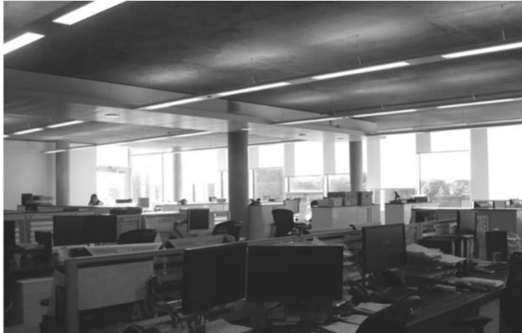
Figure 30: UK open plan office showing use of suspended ceilings and artificial lighting within a mechanically ventilated office (Shahzad S.)
