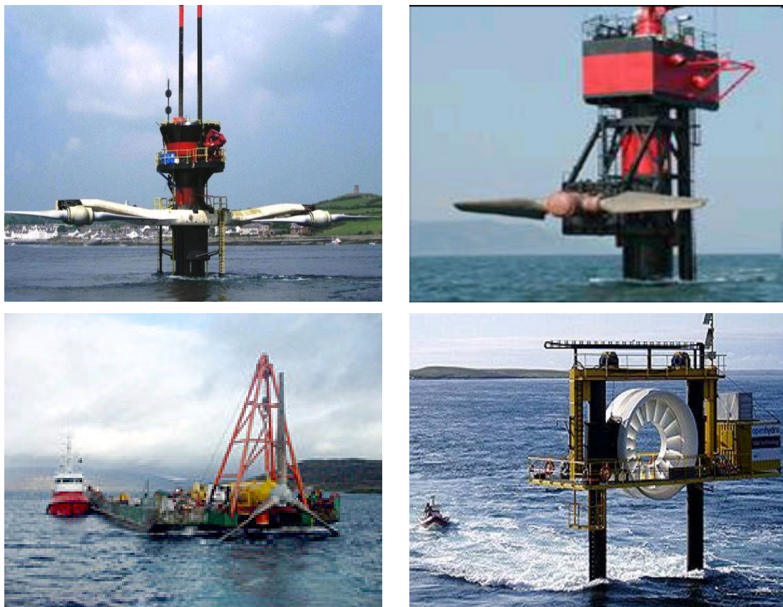
Figure 6. Clockwise from top left: SeaGen, Seaflow, Open Centre Turbine and Tidal Stream Turbine [37-39]
