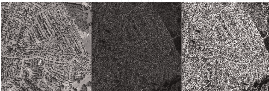
Figure 1. A montage providing an example simulation of a SAR image (the amplitude modulations) before (centre) and after (right) histogram equalisation. The simulation is based on the application of an optical image (left) using the .m code provided in Appendix A for size = 1000 and width = 3. The result is predicated on Eq. (38), where the optical image is interpreted to be a map of the self-affine variations in the dielectric properties of the ground surface.
