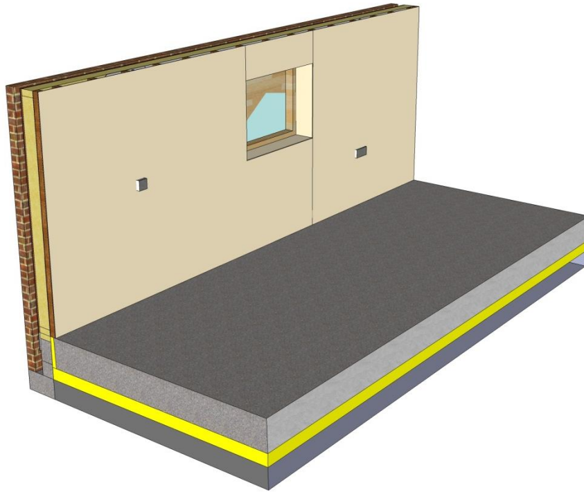
Figure 32: Image illustrating the application of plaster board and skim-coat internal wall finish
