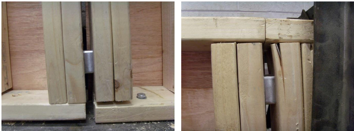
Figure 108: Images showing damage to test panels after the completion of Test 2B
