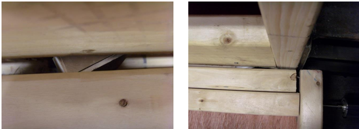
Figure 99: The left image shows pivoting Sherpa connector and the right image shows the range of movement of panel 'B' during test
