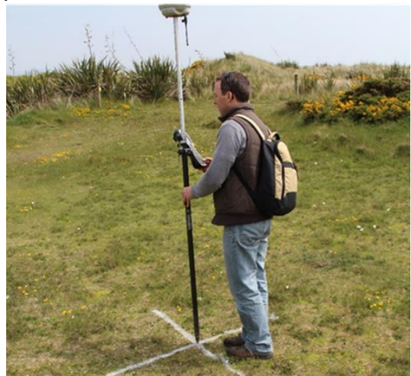
Figure 3. GCPs set on site for RPAS surveying.
