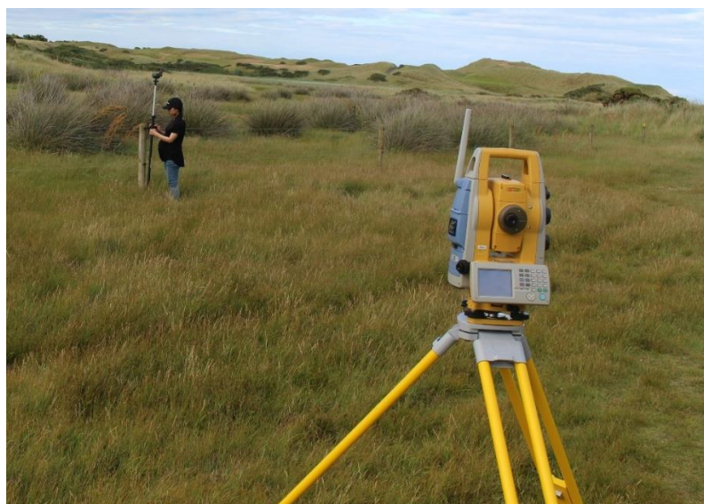
Fig.2.1 Robotic Total Station working on-site.
