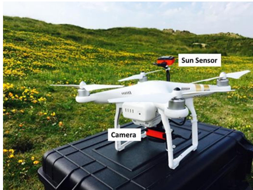
Fig.4.4 Sequoia multispectral sensor mounted on a DJI Phantom 3 Pro UAS.
