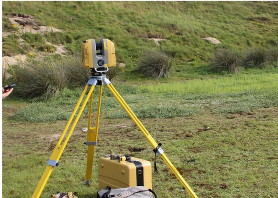
Fig.3.3 Topcon GLS2000 surveying on-site.
