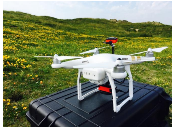
Figure 2. Sequoia multispectral sensor mounted on DJI UAS.
