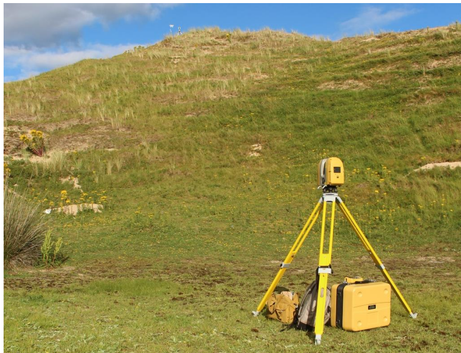
Fig.2.3 Terrestrial Laser Scanner working on-site.
