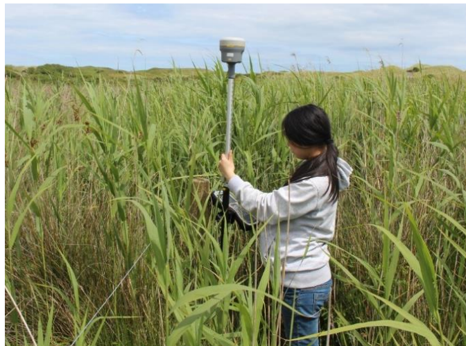
Fig.2.2 Network RTK working on-site.
