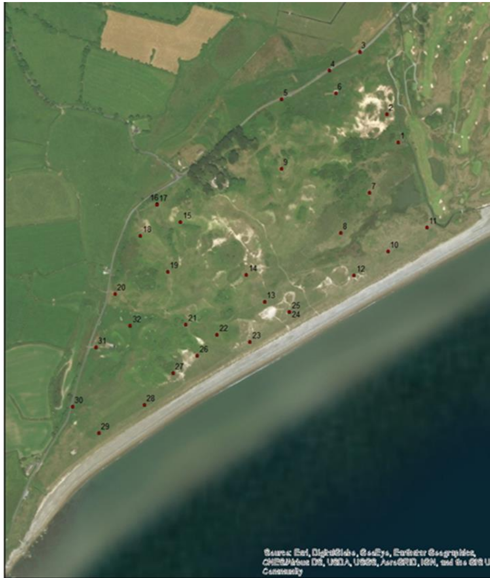
Fig. 3. Ground control points map for UAV surveying
