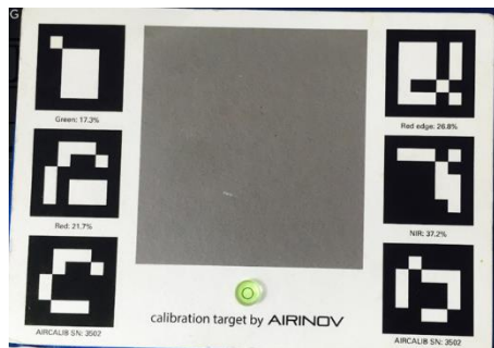
Figure 4. The balance card used for radiometric calibration.
