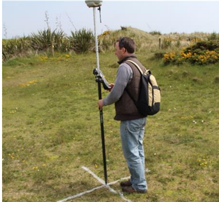
Fig.4.5 GCPs set on site for UAS surveying.
