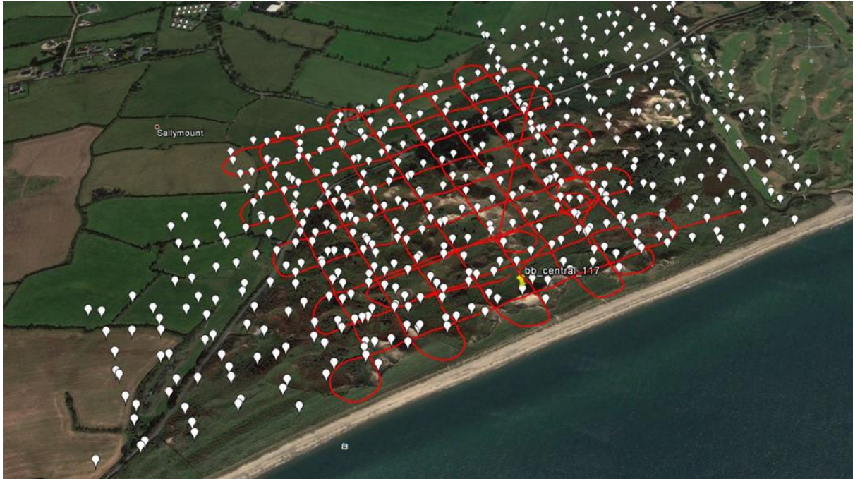
Fig. 4. Flight path for UAV surveying at three sections of study site
