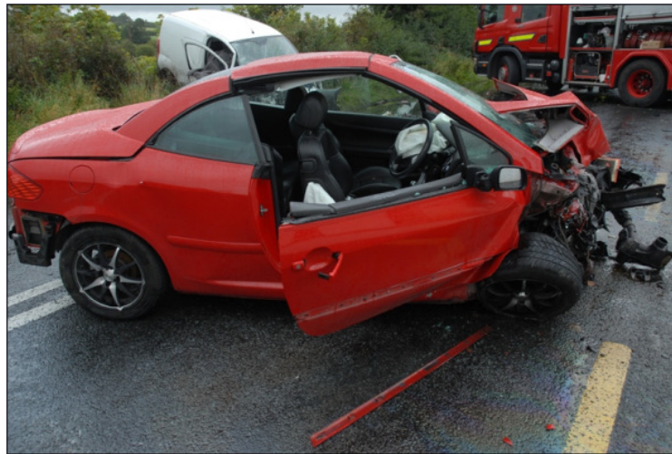
Figure 2 Vehicle Impact Absorption – Leading to Reduced Occupant’s Injuries (Peugeot Ireland)
