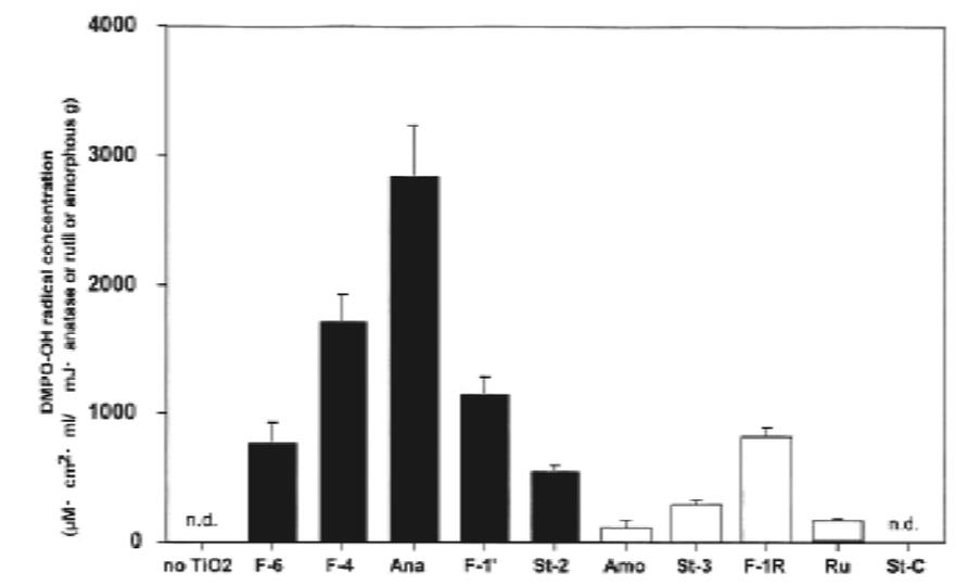
**Fig. 2: Oxidative stress hydroxyl radical production (ESR) in different TiO<sub>2</sub> polymorph phases Uchino *et al.* (2002).**
