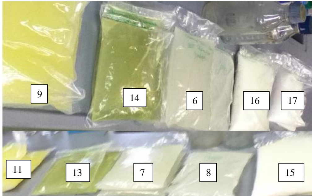
Figure 2.1 Different whey samples received from the cheese industry (Batch 4) 9: Blue cheese whey (original) pasteurised, 14: Brie cheese whey pasteurised-dialysed, 6: Cheddar cheese whey pasteurised-ultrafiltrated-permeate, 16: Skimmed milk whey pasteurised-ultrafiltrated- permeate, 17: Skimmed milk whey pasteurised- dialysed, 11: Blue cheese whey pasteurised-dialysed, 13: Brie cheese whey pasteurised-ultrafiltrated-permeate, 7: Cheddar cheese whey pasteurised-dialysed, 8: Cheddar cheese whey pasteurised-dialysed-ultrafiltrated-retentate, 15: Skimmed milk whey pasteurised-ultrafiltrated-retentate
