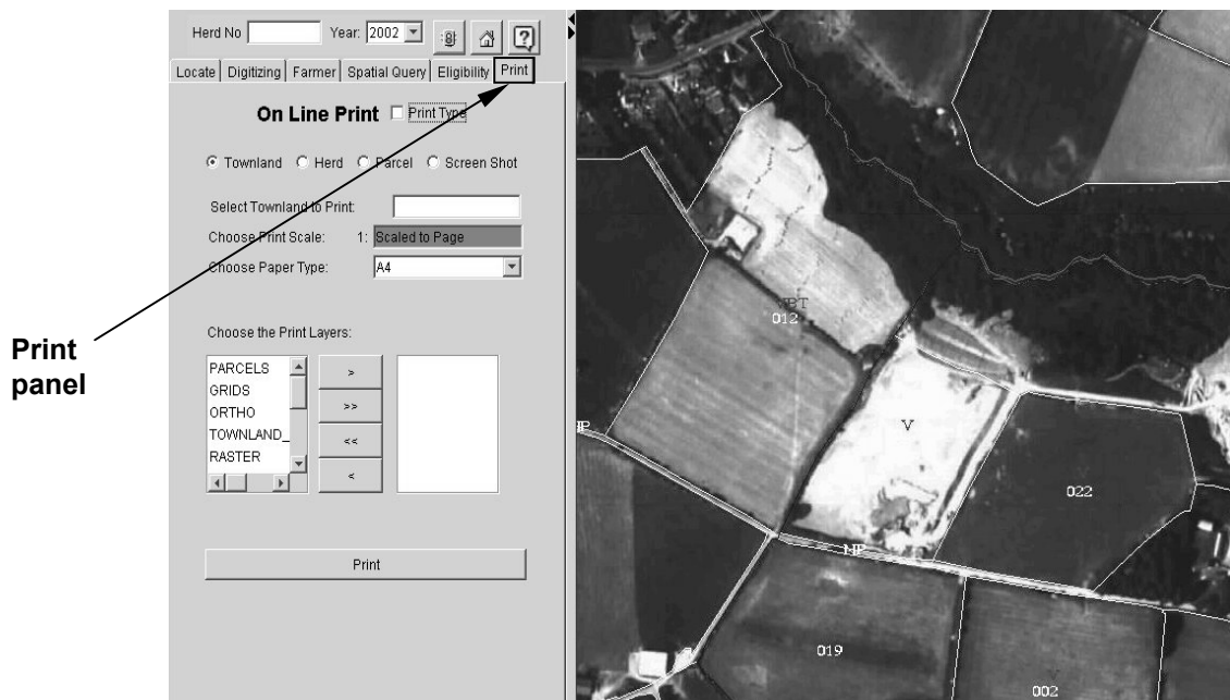
Figure 5. Printing panel with on-line option: a wide range of parameters can be selected by the user (zoom levels, paper size, background settings, etc.).
