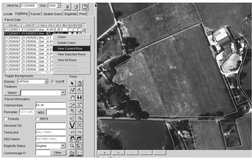
Figure 2. Alternative locate method: the user enters a herd number and year; then clicks on the Digitising tab (Parcel Data will have been populated with plot and parcel data for the chosen herd number); the specific parcel is then selected and viewed by right clicking on it and choosing the View Current Row option.
