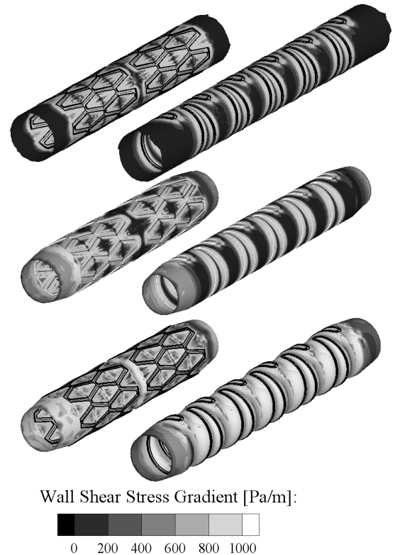
Figure 7: Contours of wall shear stress gradients for all six computational models.
