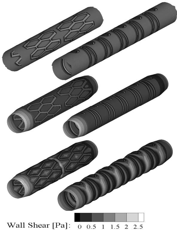
Figure 6: Contours of wall shear stress for all six computational models.
