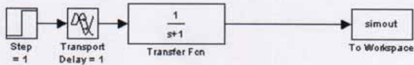
Figure (2.9) SIMULINK file with process parameters
