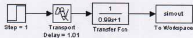
Figure (2.19) Area method process model with time delay approximation (Astrom and Hagglund (1995))
