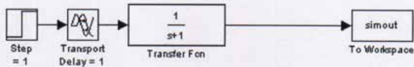
Figure (2.17) SIMULINK file with process parameters for area method algorithm
