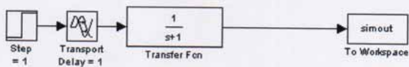
Figure (2.2) SIMULINK file with process parameters for graphical method
