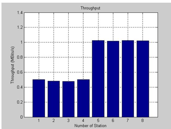
**Figure 8:** Performance of 4 TCP uploads (STAs 1-4) and 4 TCP downloads (STAs 5-8) under standard 802.11b operation, STA1-4 TCP Buffer Size equal to 32KB. STA5-8 TCP Buffer Size equal to 1MB
