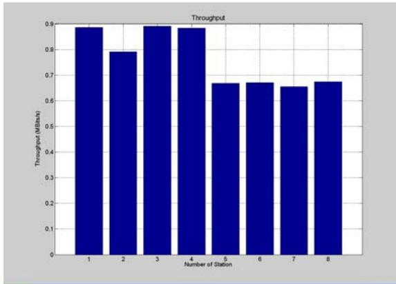
**Figure 7:** Performance of 4 TCP uploads (STAs 1-4) and 4 TCP downloads (STAs 5-8) under standard 802.11b operation. Same TCP sliding window size used in all stations (32KB).
