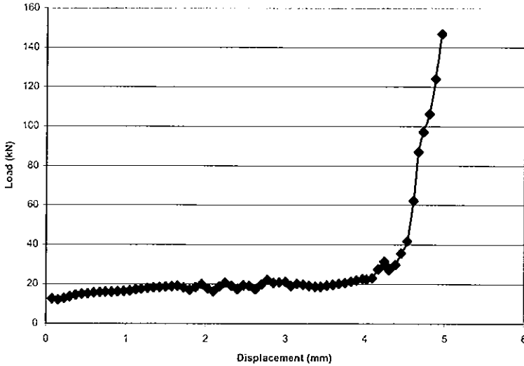
Figure 4.14 Load – Displacement 16.5 mm Die, 3.0 mm AISI 1010 (Finite Element Result)
