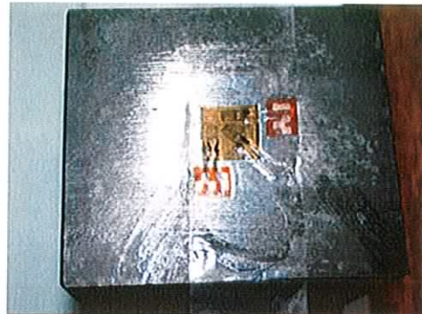
Figure 8 Strain gauge and connectors in place.
