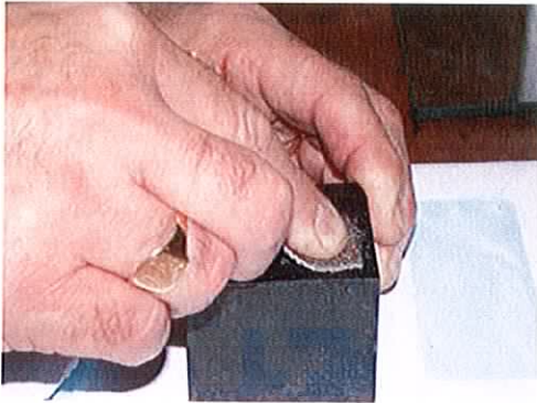
Figure 1 Abrade the tool surface to clean off any oxide from the hardening and tempering process
