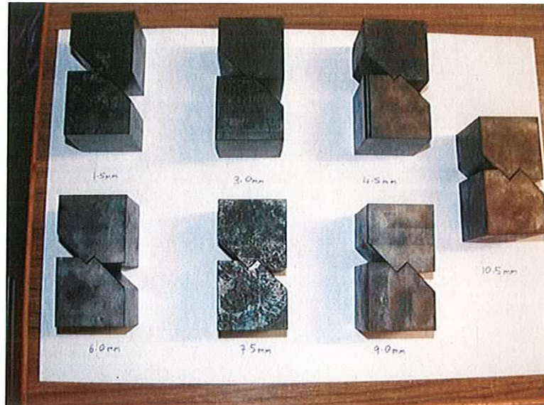
Figure 3.7. Set of tools after machining and heat treatment, prior to experimental use.
