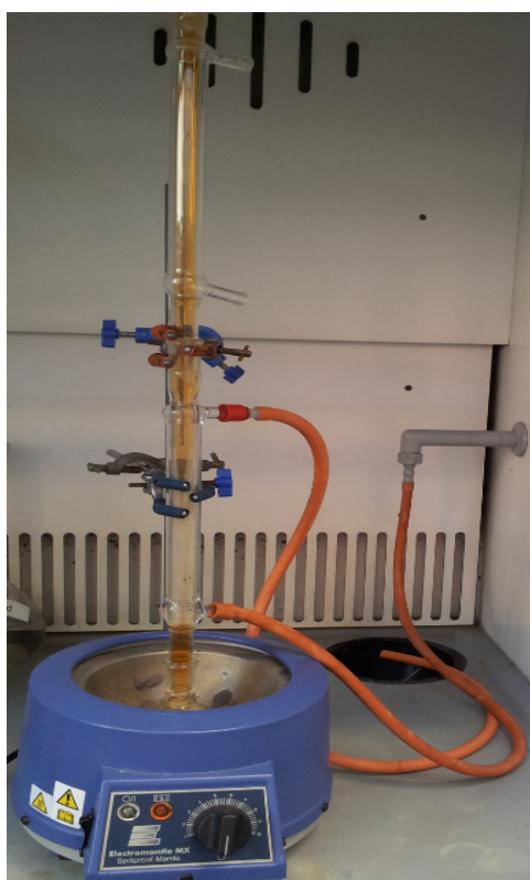
Figure 5: Reflux apparatus setup
