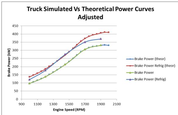
Figure 17. Sample truck engine adjusted simulated vs. theoretical power curves
