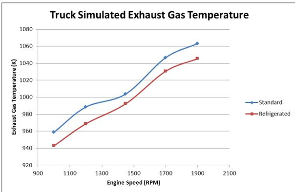
Figure 11. Sample truck engine simulated exhaust gas temperature
