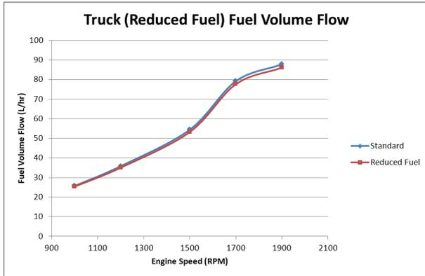
Figure 21. Sample truck engine (reduced fuel) simulated fuel volume flow
