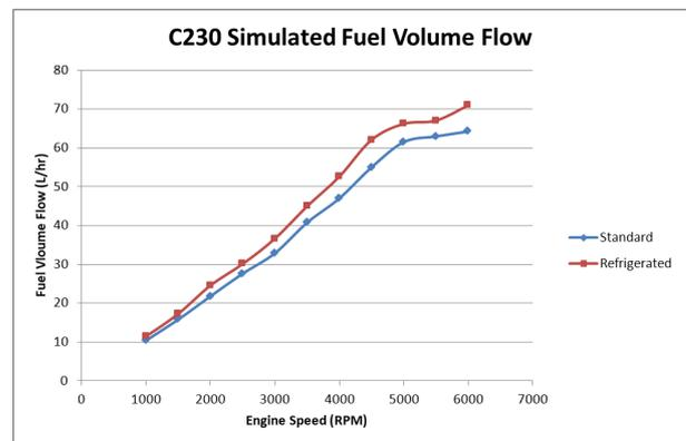
Figure 8. C230 engine simulated fuel volume flow
