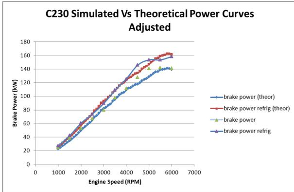
Figure 13. C230 engine adjusted simulated vs. theoretical power curves
