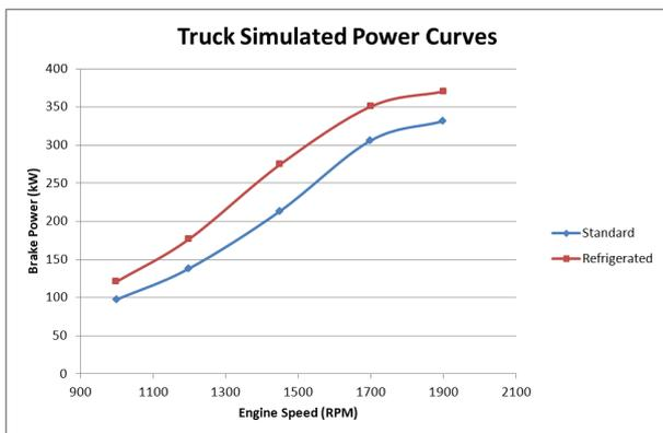
Figure 5. Sample truck engine simulated power curves
