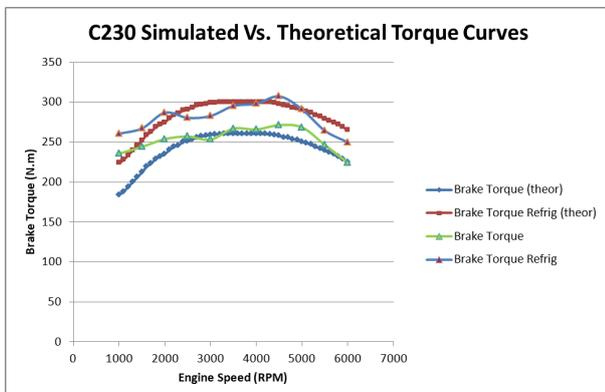
Figure 14. C230 engine simulated vs. theoretical torque curves
