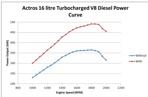
Figure 2. Actros engine power curves
