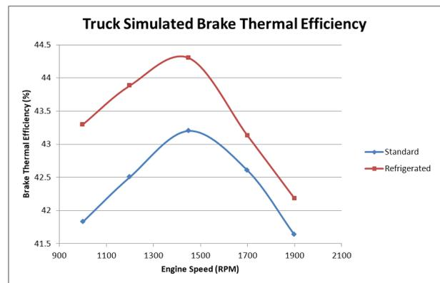
Figure 7. Sample truck engine simulated brake thermal efficiency
