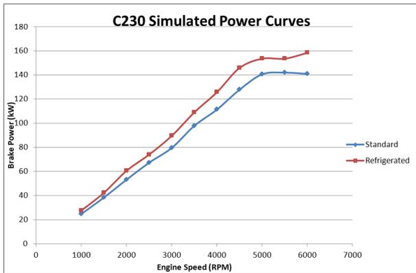
Figure 4. C230 engine simulated power curves
