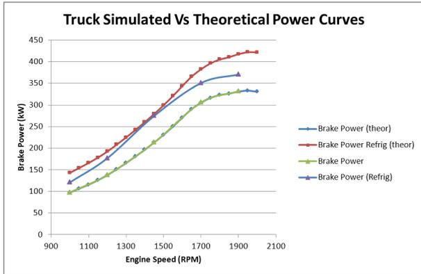
Figure 16. Sample truck engine simulated vs. theoretical power curves
