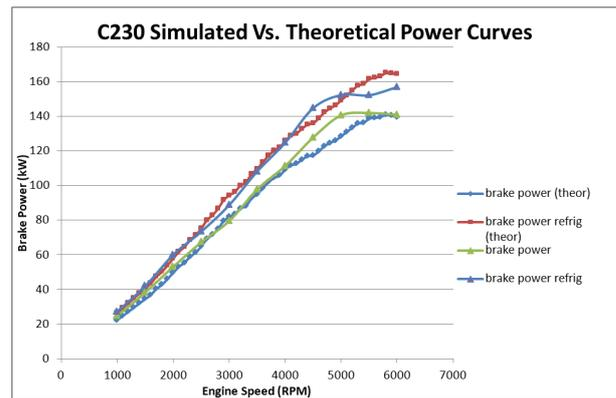
Figure 12. C230 engine simulated vs. theoretical power curves
