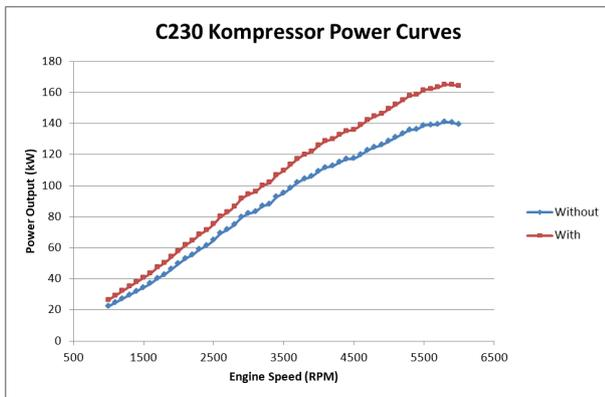
Figure 1. C230 engine power curves
