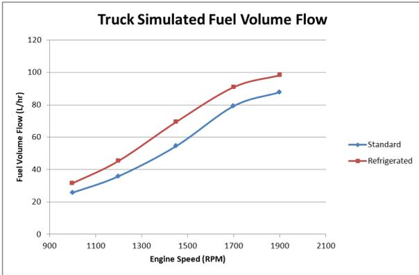
Figure 9. Sample truck engine simulated fuel volume flow
