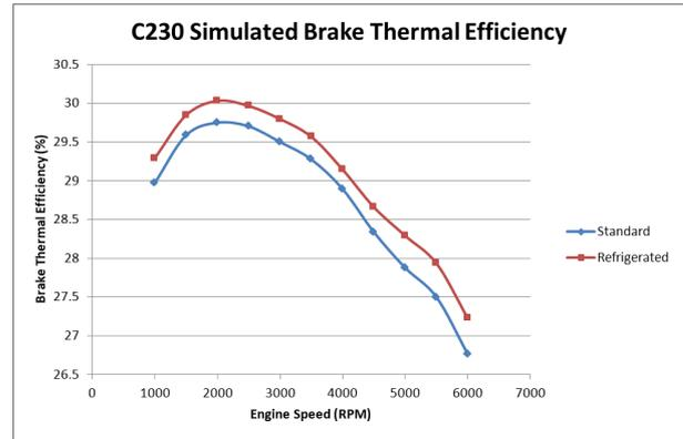
Figure 6. C230 engine simulated brake thermal efficiency
