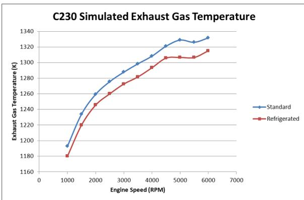
Figure 10. C230 engine simulated exhaust gas temperature
