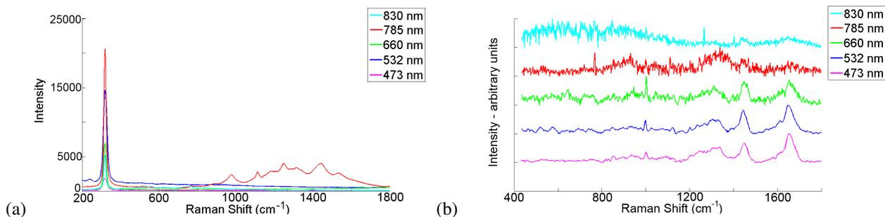
**Fig. 6** (a) Background signal of **IR polished calcium fluoride** recorded for each of the above wavelengths, (b) normalised Raman signals from cells recorded on IR polished calcium fluoride for each of the above wavelengths, with an acquisition time of 30 s (x2).
