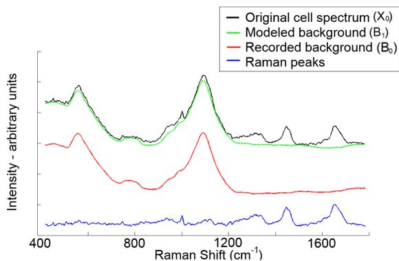
**Fig. 2** An example of how the background subtraction algorithm works - whereby the recorded background signal is combined with a fifth order polynomial until a value of  $C$  is found such that the modeled background fits directly under the Raman peaks of the original cell spectrum.
