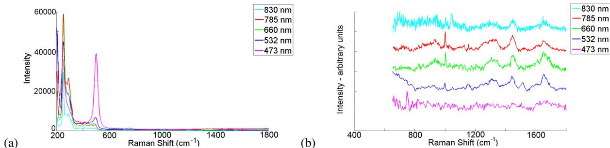
**Fig. 14** (a) Background signal of **zinc selenide** recorded for each of the above wavelengths, (b) normalised Raman signals from cells recorded on zinc selenide for each of the above wavelengths, with an acquisition time of 30 s (x2). Note, the cell spectra are only shown between 600–1800  $\text{cm}^{-1}$  due to the large background contribution in the lower wavenumber region.
