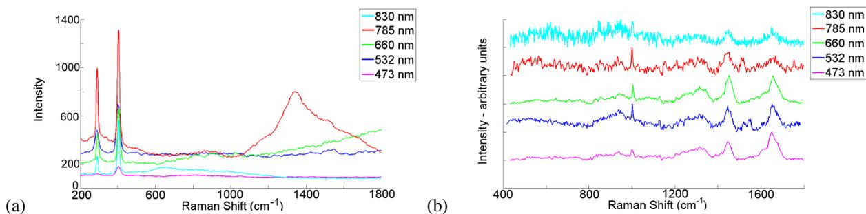
**Fig. 11** (a) Background signal of **magnesium fluoride** recorded for each of the above wavelengths, (b) normalised Raman signals from cells recorded on magnesium fluoride for each of the above wavelengths, with an acquisition time of 30 s (x2).
