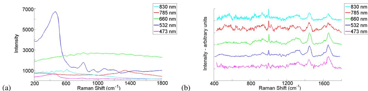
**Fig. 9** (a) Background signal of **1500 nm aluminium thin film on glass** recorded for each of the above wavelengths, (b) normalised Raman signals from cells recorded on 1500 nm aluminium thin film for each of the above wavelengths, with an acquisition time of 30 s (x2).
