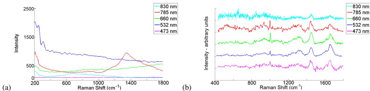
**Fig. 12** (a) Background signal of **potassium bromide** recorded for each of the above wavelengths, (b) normalised Raman signals from cells recorded on potassium bromide for each of the above wavelengths, with an acquisition time of 30 s (x2).
