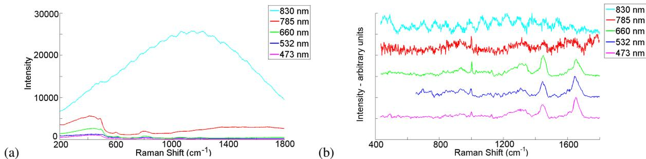
**Fig. 7** (a) Background signal of **fused silica** recorded for each of the above wavelengths, (b) normalised Raman signals from cells recorded on fused silica for each of the above wavelengths, with an acquisition time of 30 s (x2). Note, the cell spectrum at 532 nm is only shown between 600-1800  $\text{cm}^{-1}$  due to the large background contribution in the lower wavenumber region.
