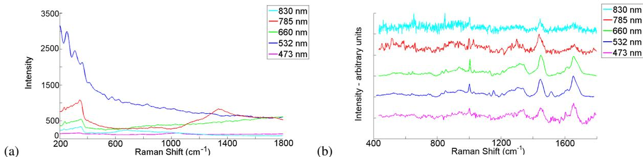
**Fig. 13** (a) Background signal of **sodium chloride** recorded for each of the above wavelengths, (b) normalised Raman signals from cells recorded on sodium chloride for each of the above wavelengths, with an acquisition time of 30 s (x2).
