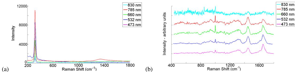
**Fig. 5** (a) Background signal of **Raman-grade calcium fluoride** recorded for each of the above wavelengths, (b) normalised Raman signals from cells recorded on Raman-grade calcium fluoride for each of the above wavelengths, with an acquisition time of 30 s (x2). Note, improved spectra at 830 nm can be obtained using a longer acquisition time.
