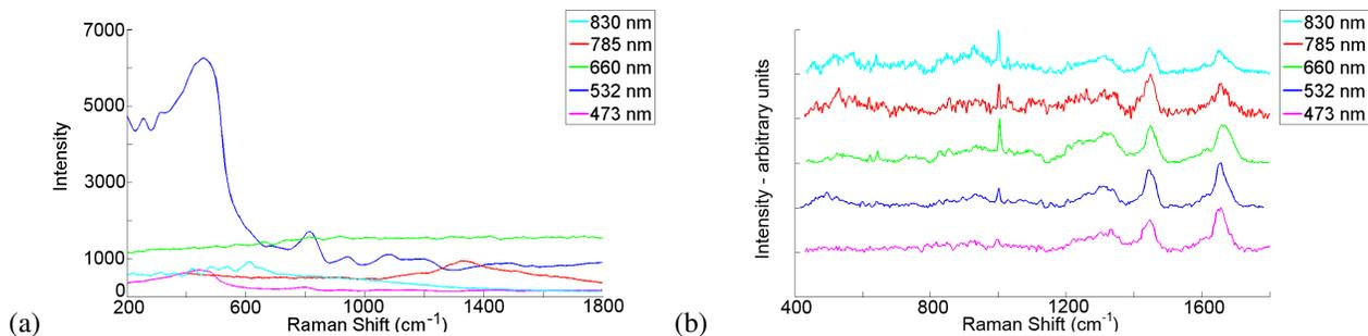
**Fig. 8** (a) Background signal of **100 nm aluminium thin film on glass** recorded for each of the above wavelengths, (b) normalised Raman signals from cells recorded on 100 nm aluminium thin film for each of the above wavelengths, with an acquisition time of 30 s (x2).
