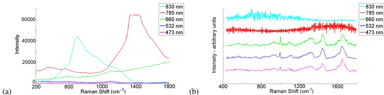
**Fig. 10** (a) Background signal of **glass** recorded for each of the above wavelengths, (b) normalised Raman signals from cells recorded on glass for each of the above wavelengths, with an acquisition time of 30 s (x2). Note, the recorded background signal at 785 nm saturated in the  $1400\text{ cm}^{-1}$  region.
