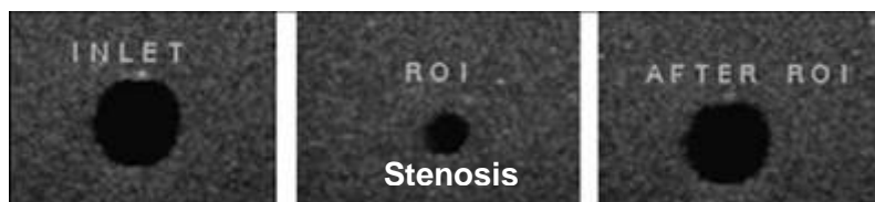
360 Figure 8 Transverse views of a phantom with a 50% stenosis at the position of (a) 10 mm after the inlet, (b) the stenosis and (c) 10 mm before the bend.
