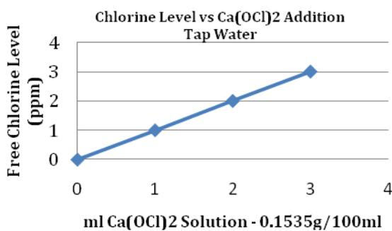
Figure 4 – Chlorine Level vs Calcium Hypochlorite Addition
