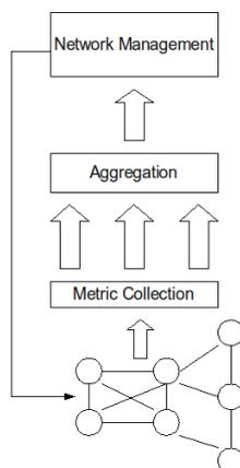
**Figure 1: Network parameter modification using QoS metric aggregation.**
