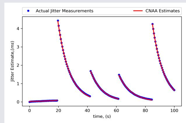
**Figure 5.** Accuracy of the CNA prediction model: The obtained predictions are overlaid on the jitter measurements.
