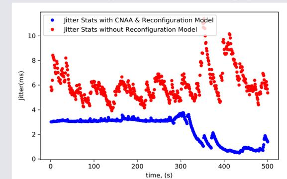
**Figure 6.** Effect of the CNA agent estimations and the SDN reconfiguration component: We record a 64% performance improvement in the jitter statistics.
