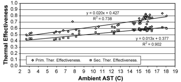
Fig. 2. Variation in thermal effectiveness with typical annual range of AST in Dublin (load 20 kW, flow rates: tower water flux 2.9 kg/s m<sup>2</sup>, tower air flux 4.0 kg/s m<sup>2</sup>, secondary water 1.6 kg/s).
