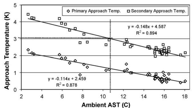
Fig. 3. Variation in primary and secondary approach temperature with annual range of AST in Dublin (load 20 kW, flow rates: tower water flux 2.9 kg/s m<sup>2</sup>, tower air flux 4.0 kg/s m<sup>2</sup>, secondary water 1.6 kg/s). The mean AST of 10.5 °C is shown with associated 3 K SAT.
