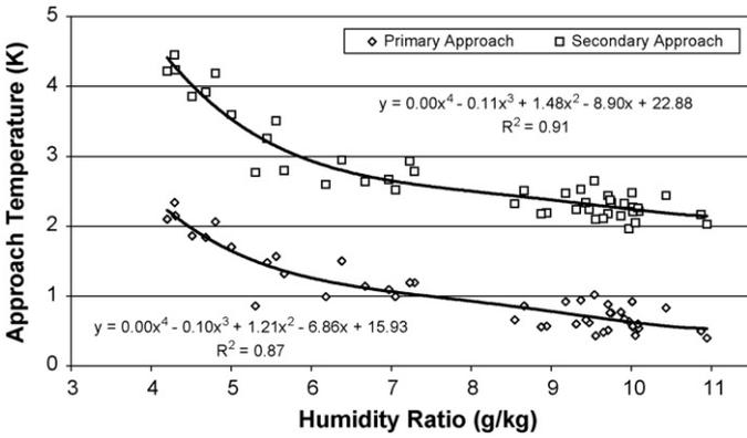
Fig. 6. Polynomial variation in primary and secondary approach temperature with annual range of humidity ratio (as the DBT varies) in Dublin (load 20 kW, flow rates: tower water flux 2.9 kg/s m<sup>2</sup>, tower air flux 4.0 kg/s m<sup>2</sup>, secondary water 1.6 kg/s).
