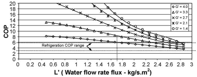
Fig. 8. Results of analysis of COP of the test rig as a function of the air-flow rate flux ( $G'$ , kg/s m<sup>2</sup>) and the water-flow rate flux ( $L'$ , kg/s m<sup>2</sup>). The range of total power input COP possible with vapour compression refrigeration (2.6–5.7) is also shown.
