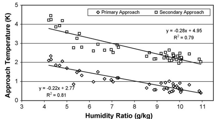
Fig. 5. Linear variation in primary and secondary approach temperature with annual range of humidity ratio (as the DBT varies) in Dublin (load 20 kW, flow rates: tower water flux 2.9 kg/s m<sup>2</sup>, tower air flux 4.0 kg/s m<sup>2</sup>, secondary water 1.6 kg/s).
