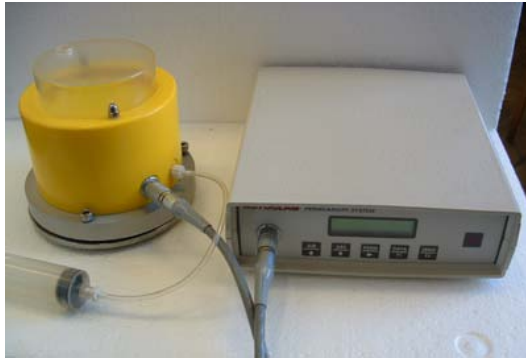
Fig. 4a Autoclam Permeability System, with bonding type base ring
