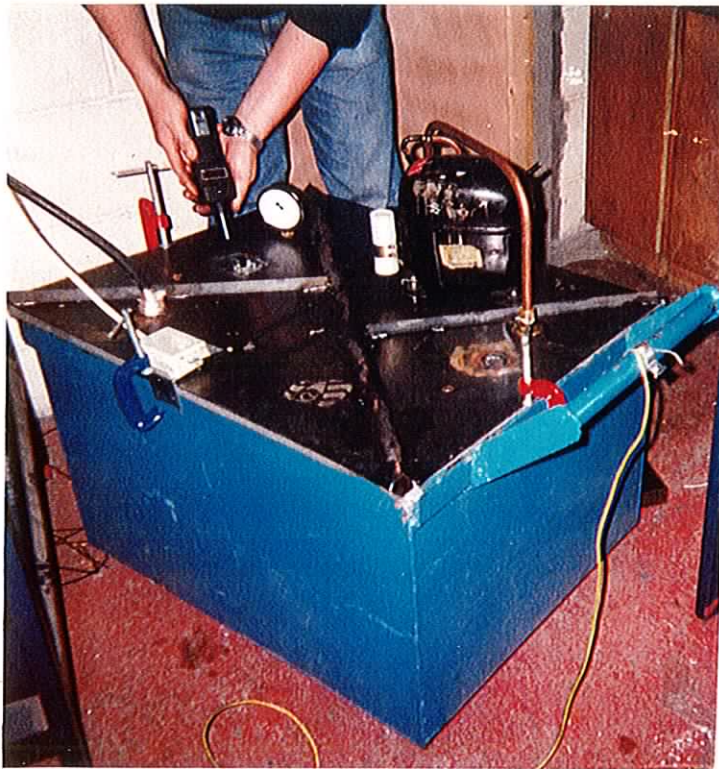
Figure 4.8 Reinforced box top with a window aperture for flywheel speed measurement and with other interfaces for the vacuum pump, pressure gauge and electrical connections to the motor
