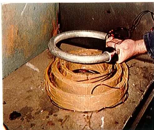
Figure 2.8c The ring flywheel over 3 hollow iron cores with interspersed windings--one of the iron-based approaches to realising a stable bearing arrangement
