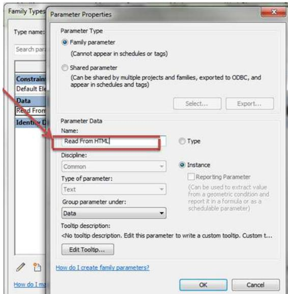
Fig. 3: Custom parameter properties added to the family to enable energy readings to be fed into the family data.
