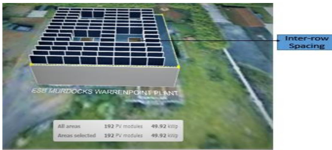
Figure 4. The PV system simulation description of a grid-connected solar system of ESB Murdocks Warrenpoint Plant ( https://www.sunnydesignweb.com/sdweb/#/Home ).
