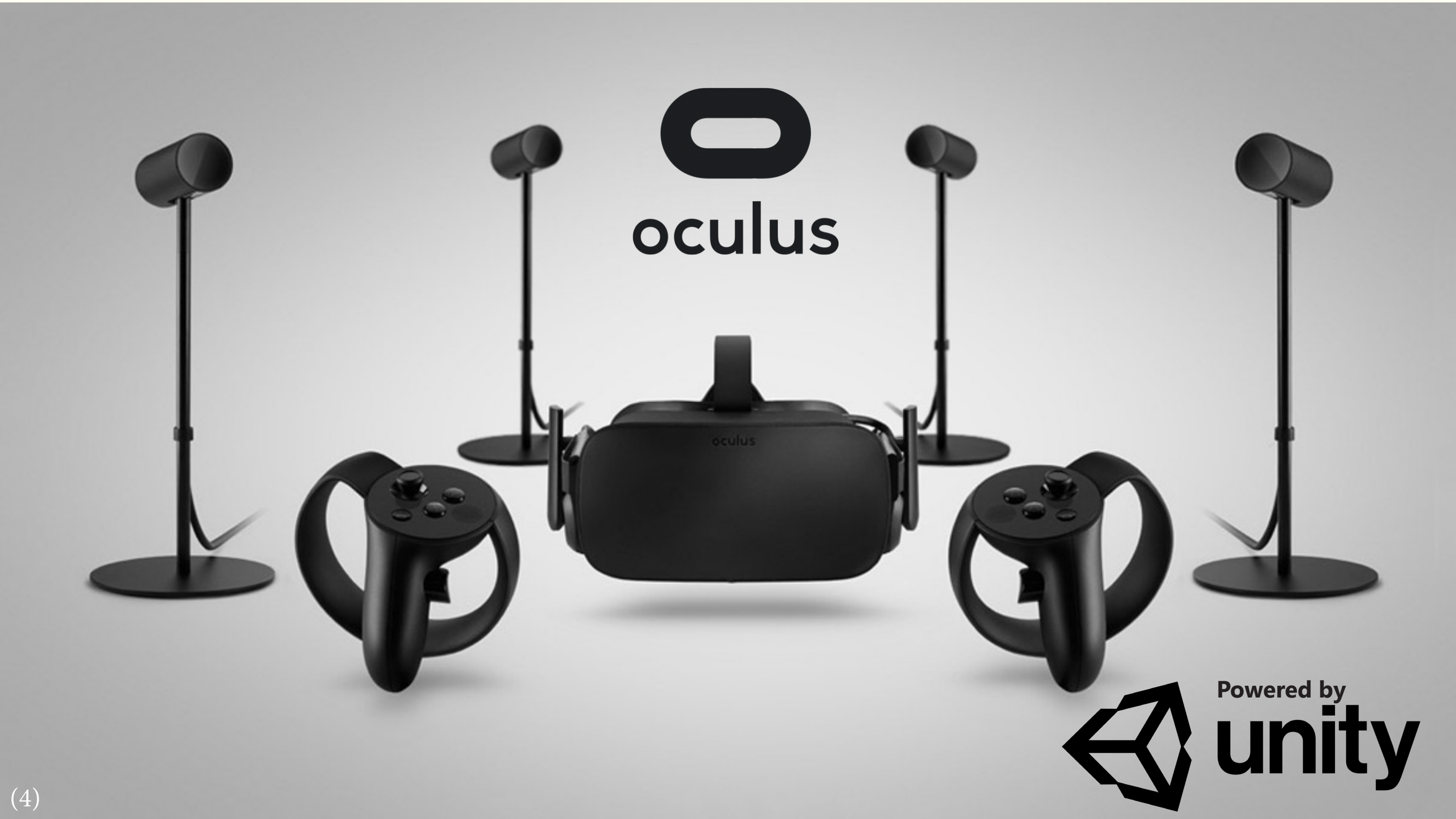
(4) iAn Oculus Rift Touch Virtual Reality headset. The Main headset allows a viewer to experience a 3D environment, in this case a 3D model of a human brain and associated tractography. Two controllers, one in each hand, allow manipulation of the scene and selecting/deselecting tracts for easier visualisation. The four trackers allow for extremely accurate tracking of the viewer's head and hand movements. (4.1) Unity 3D logo - Unity 3D was the primary software utilised to create the virtual reality environment for tractography visualisation, as well as to provide user feedback through visual and audio cues.
