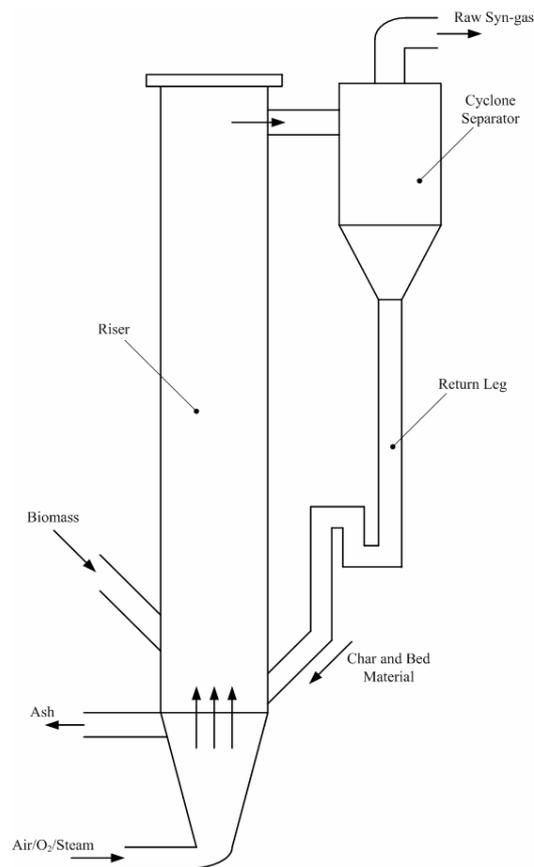
Fig. 1. Schematic diagram of a CFB biomass gasifier.
