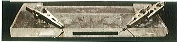
Figure 4.6: Mount used to hold PV cell in position for electrical measurements
