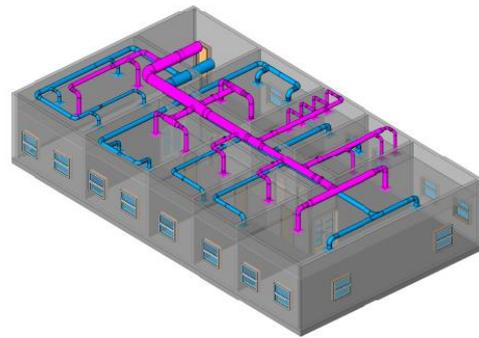
Fig. 1: The Revit model with HVAC system
