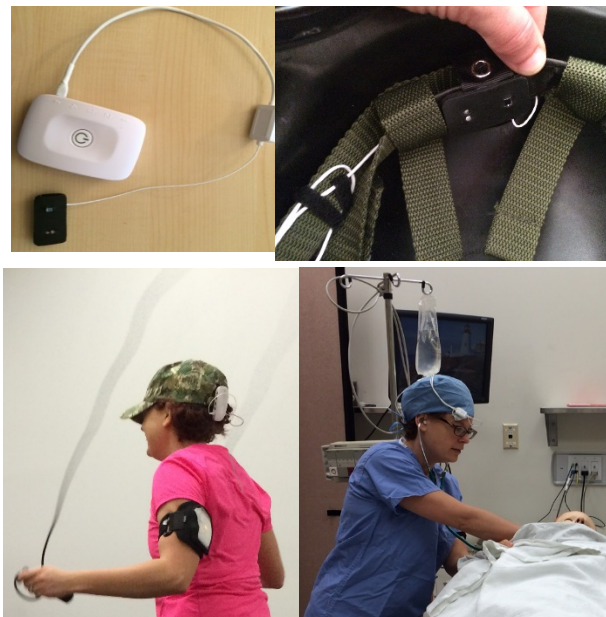
Fig. 1. Custom fNIRS sensor alone (top left), mounted inside a helmet (top right), worn during jump roping (bottom left), and worn during a medical training simulation (bottom right)
