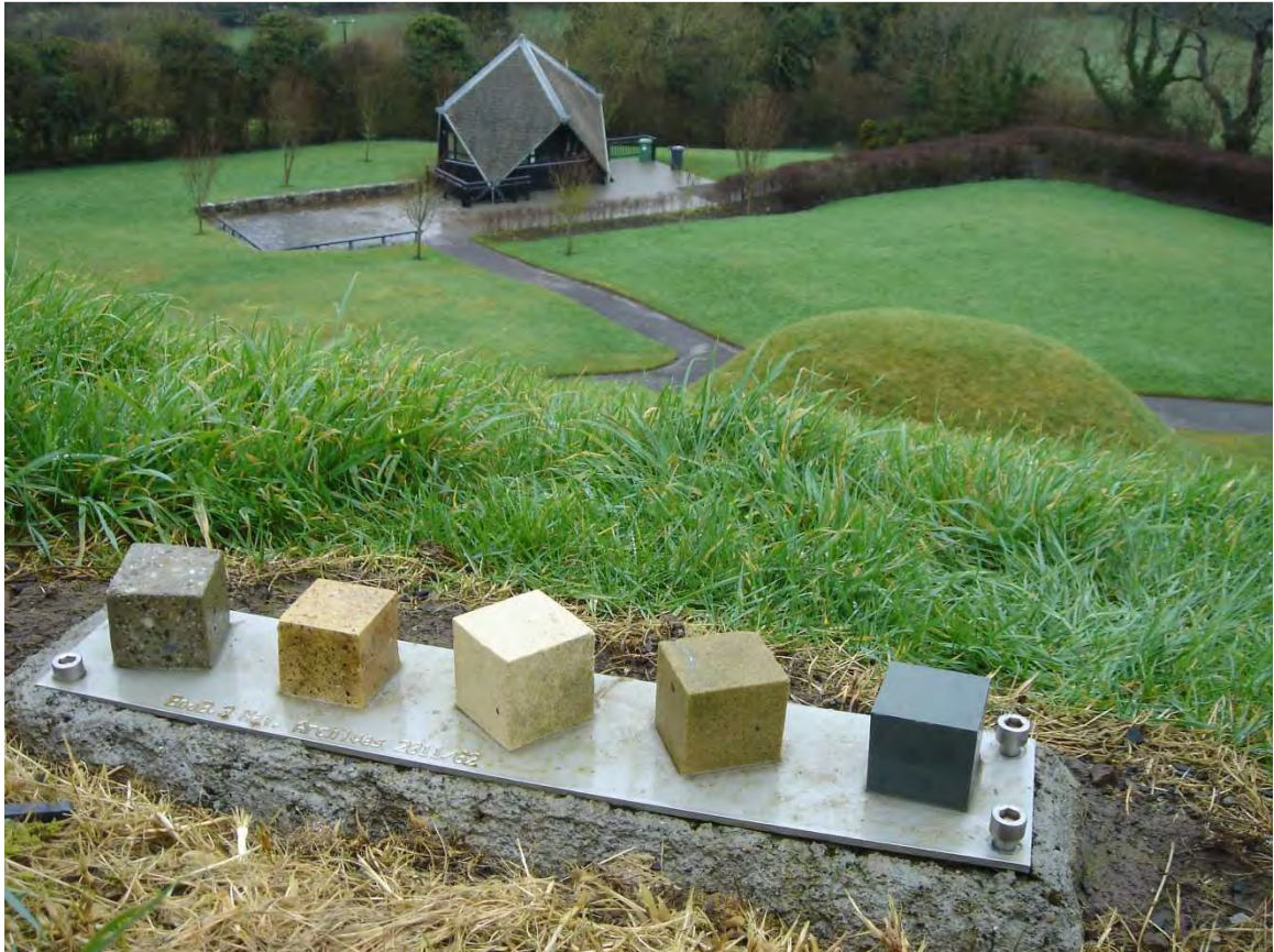
Figure 10.15. Brú na Bóinne plate No. 3 (BnB3) (Knowth) showing variance in orientation of cubes after one year exposure, February 2013
