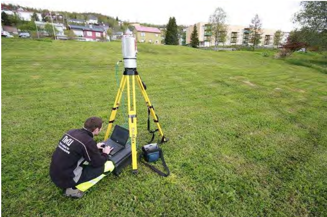
Figure 5.23. 3D laser scanning of Saurbekken farm mound, Troms (Martens 2012)
