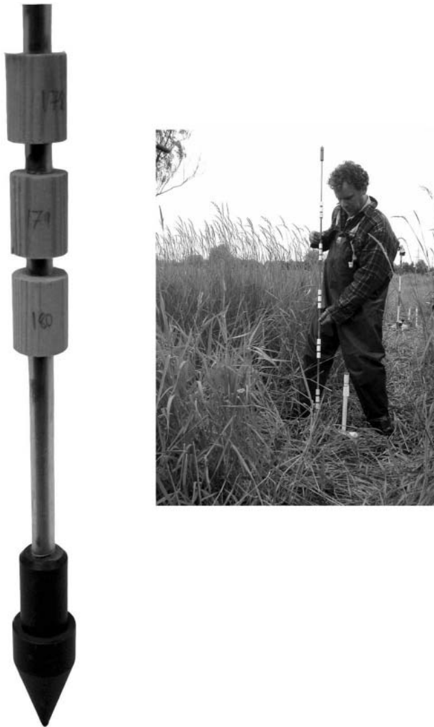
Figure 9.5. Close up of prepared wood samples on spiked rod and complete set prepared for insertion in soil (Gregory et al., 2008)
