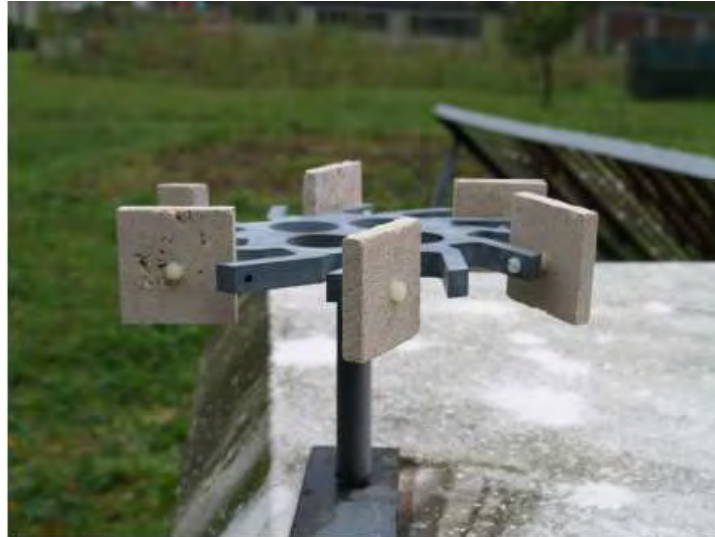
Figure 10.2. International Co-operative Programme (ICP) stone test samples on rotating carousel, Katowice, Poland (Tidblad, 2009)
