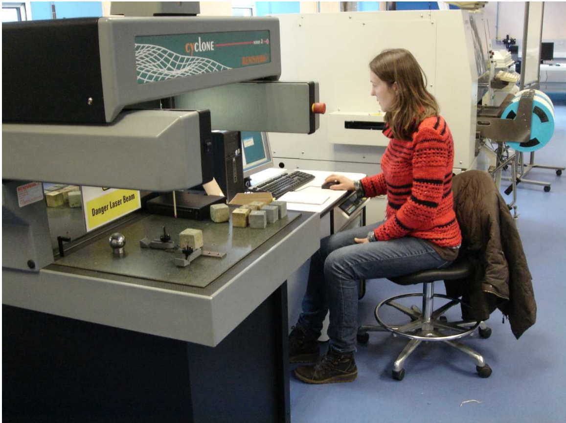
Figure 10.12. Conducting 3D profile measurements with Renishaw Cyclone Series 2 SP600M, Dublin Institute of Technology, April 2013
