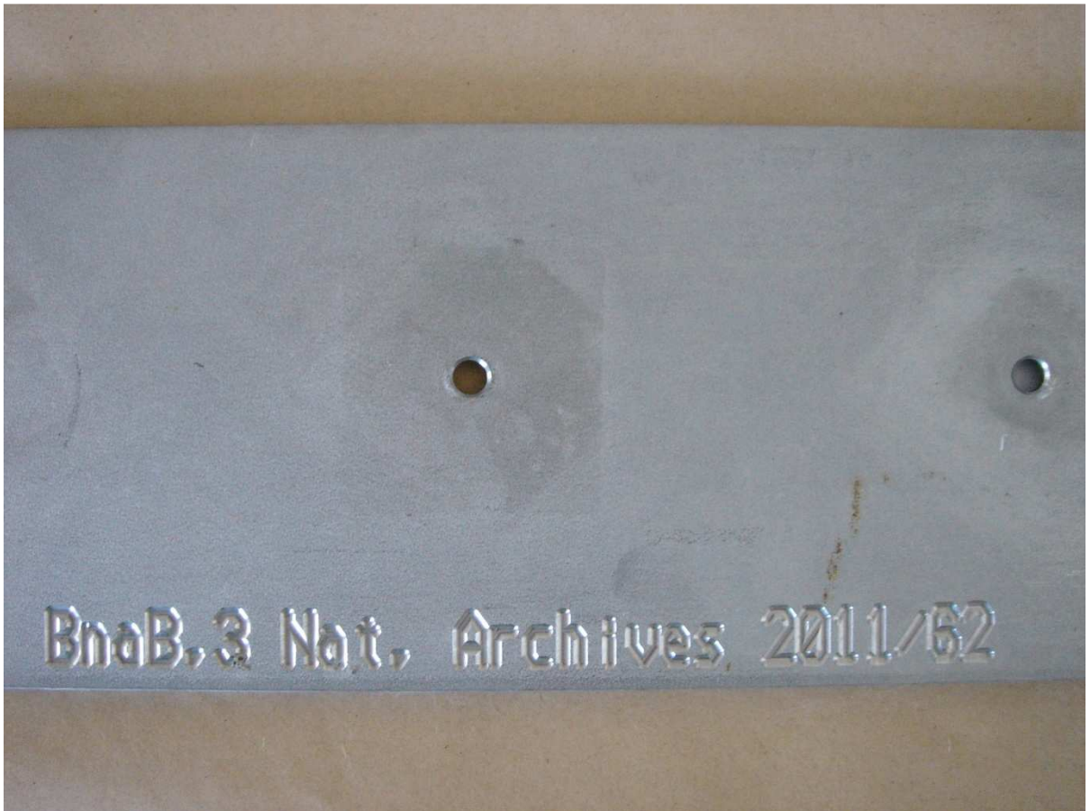
Figure 10.13. Engraved label on Brú na Bóinne stainless steel plate: abbreviated site name (BnB), plate number (3) and National Archives reference number (2011/62)
