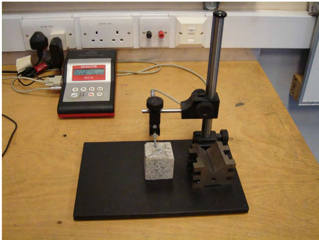
Figure 10.11. Set up for surface roughness measurement with the Diavite DH-6, Dublin Institute of Technology, April 2013
