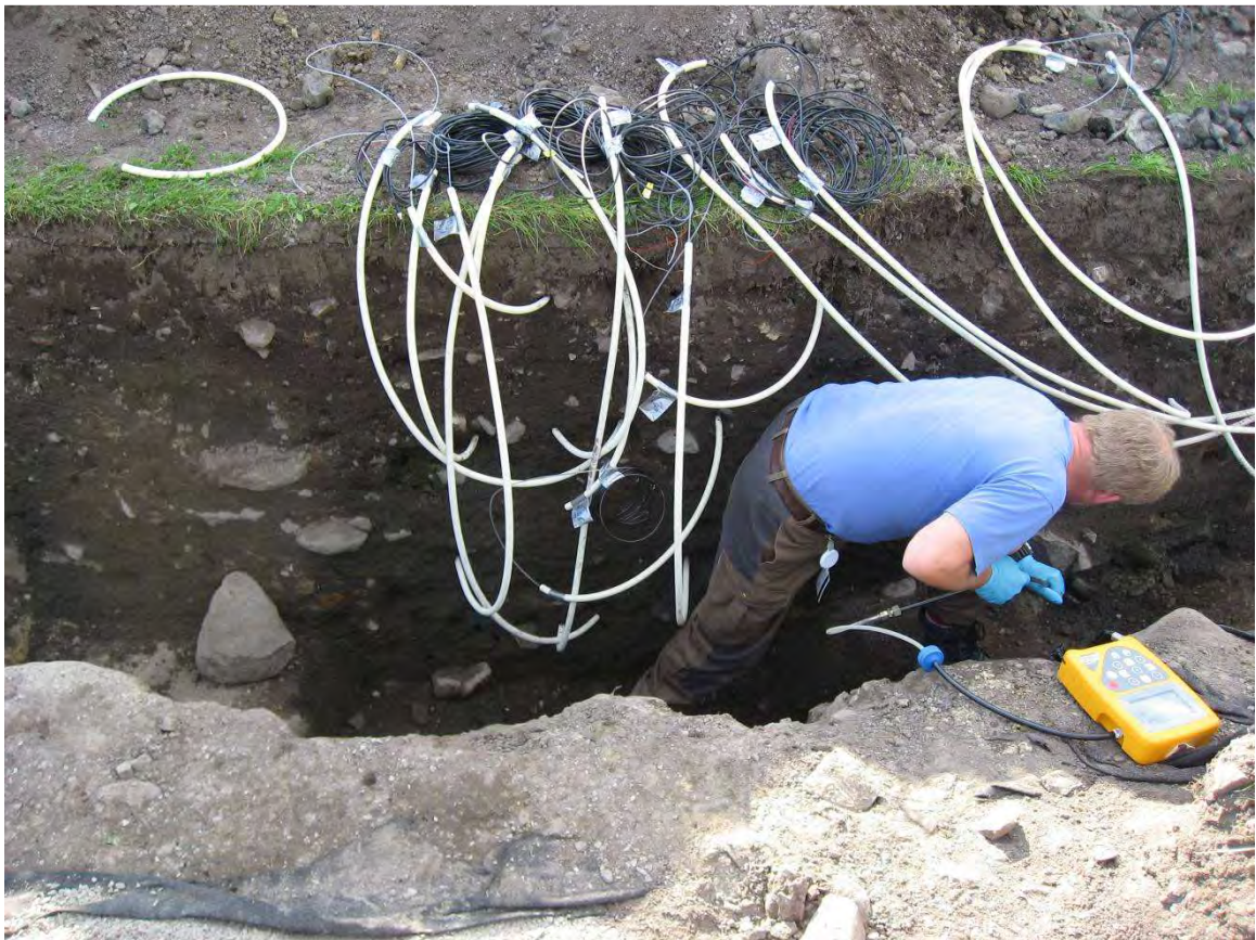
Figure 5.21. Installing monitoring equipment at Åker gård, Hamar, Hedmark; probes measuring soil temperature and water content (Martens 2007) working in section allows exact placement of probes within the stratigraphy
