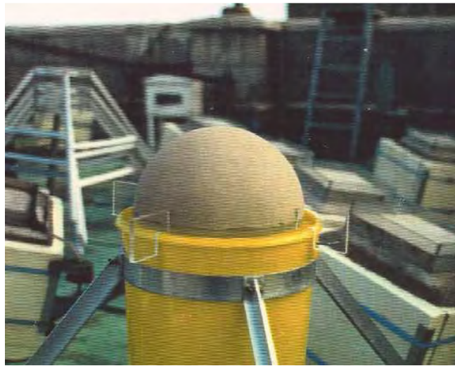
Figure 10.4. Limestone sample and runoff catchment unit, STEP programme, Trinity College Dublin (Cooper et al., 1991)
