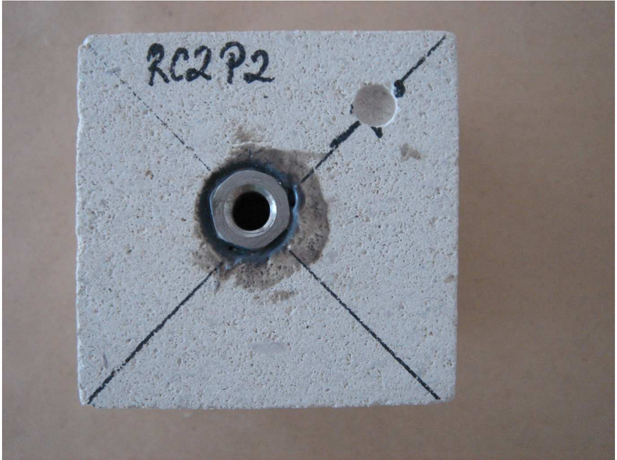
Figure 10.22. Base of cube showing sunken stainless nut and drilled reference point (top right corner) suggested control points for future 3D scanning.
