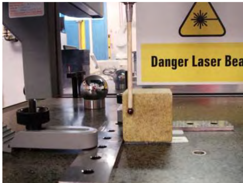
Figure 10.10. Set up for 3D profile scanning using touch probe, Dublin Institute of Technology, April 2013
