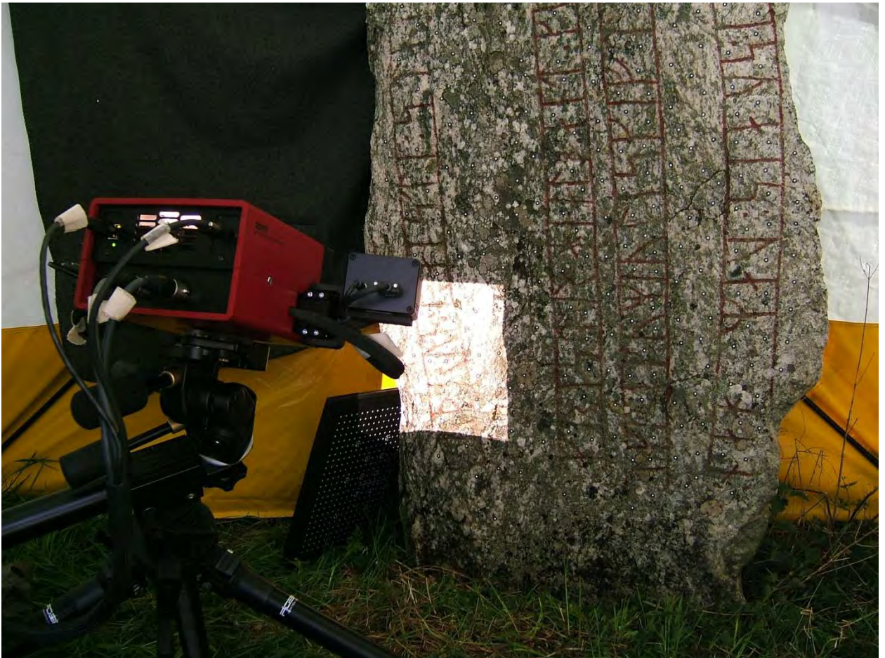
Figure 5.18. 3D scanning in progress; reference point stickers are placed on the stone to enable the software to knit individual sections together (Daly 2012).
