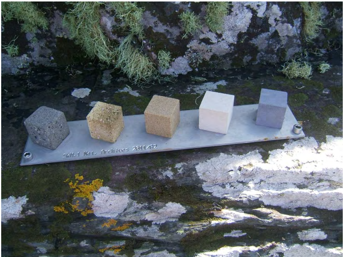
Figure 10.6. Skellig Michael LegIT plate No. 1 in situ , from left to right: concrete, brick, Peakmoor, Portland, Old Red Sandstone (August 2013)
