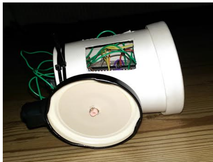
Figure 1. Sample Robot. This figure illustrates an example robot constructed with a take-away soup cup chassis and jam jar lid wheels.
