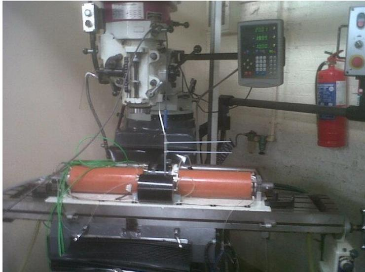
Fig 3. 3 axis experimental set up to map magnetic field
