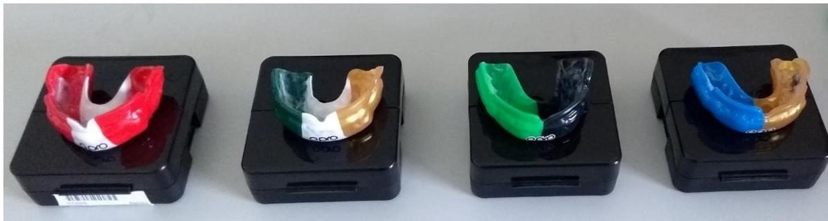
Figure 2: CAMLab Instrumented mouthguard
