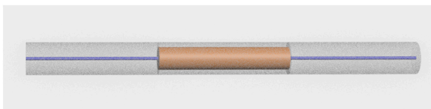
Figure 1. Schematic configuration of an SMS fiber structure [22]. Reproduced with permission from Xianfan Wang, Elfed Lewis, Pengfei Wang, Investigation of the Self-Imaging Position of a Singlemode-Multimode-Singlemode Optical Fiber Structure; published by Wiley Online Library, 2017.
