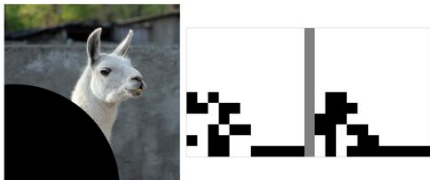
Figure 5: Example of the bit-errors generated in both the Red and Blue channels (right) by the partial removal of a portion of the watermarked image as shown (left). The rest of the image on the right-hand-side is white indicating that there are no bit-errors in the remaining portion of the watermark after extraction from the spoiled image. This is due to the BCH error correcting code that is applied which easily compensates for the data corruption shown, the remainder of the watermark in the image being extracted without bit errors.
