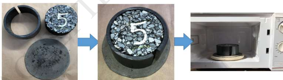
Figure 3. Microwave healing test system set up.
