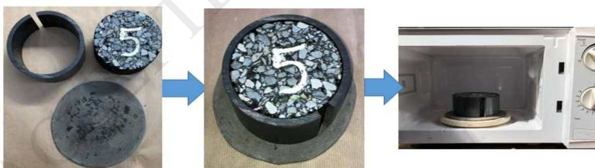
Figure 3. Microwave healing test system set up.
