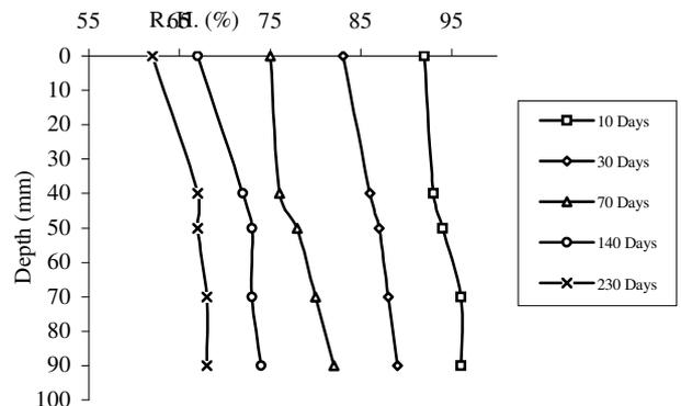
Figure 13: Pore humidity at various depths over time in the laboratory.
