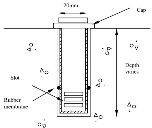
Figure 3: Drilled hole with slotted tube in place for CE-RH readings.
