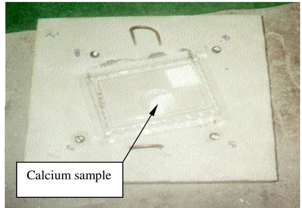
Figure 7: VET set-up showing the calcium chloride sample in the sealed tent.
