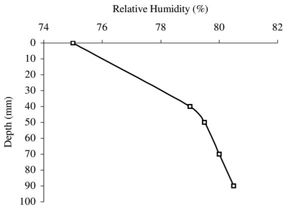
Figure 1: Typical residual moisture in a slab when the surface is at 75% RH.
