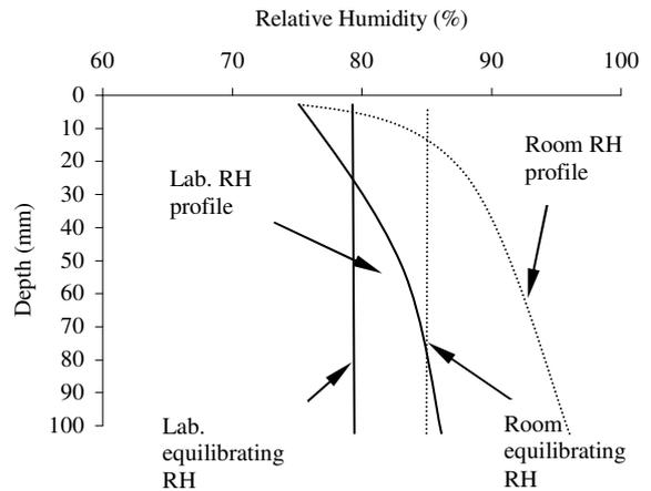
Figure 15: Effect of applying floor covering too early, with forced drying.
