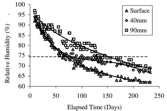
Figure 11: Variation of relative humidity with time for different depths in the laboratory sample.
