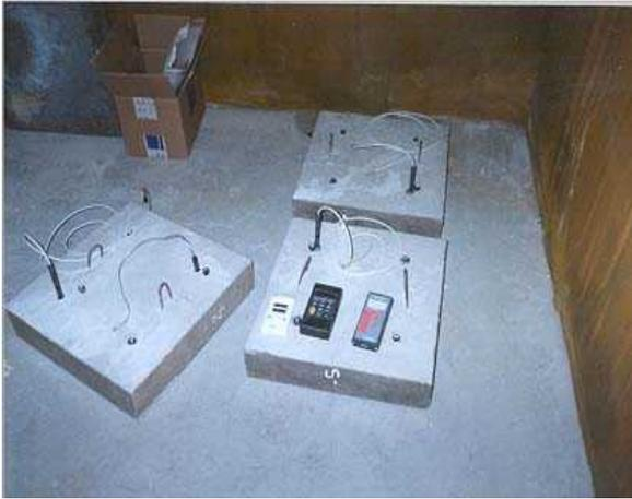
Figure 4: The complete experimental set-up showing the humidity probes, CE-RH and the CME.
