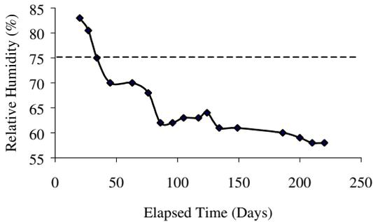
Figure 9: Surface hygrometer variation with time for the laboratory sample.
