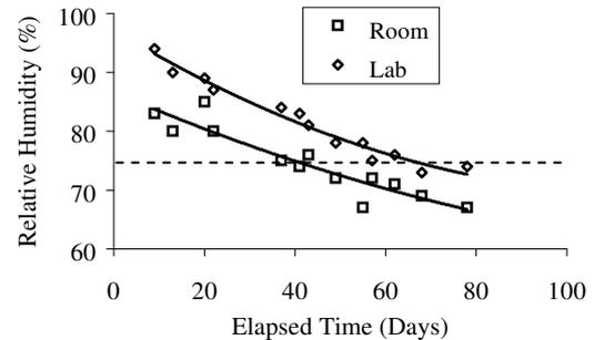
Figure 12: Variation in surface RH reading with time for slabs under different drying conditions (CE-RH).
