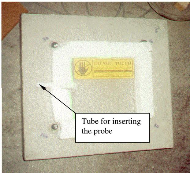
Figure 5: Surface RH apparatus with sealed tent: The humidity probes inserts into the tube on the left.
