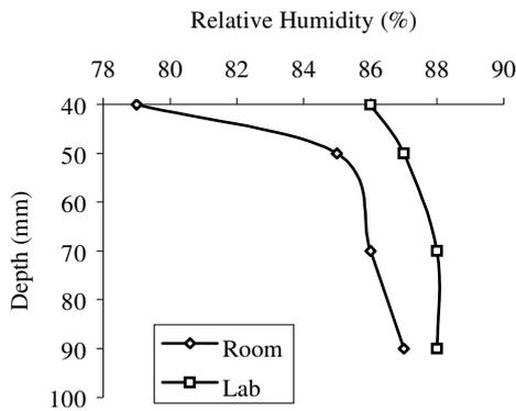
Figure 14: Moisture condition due to different drying condition at 28 days.
