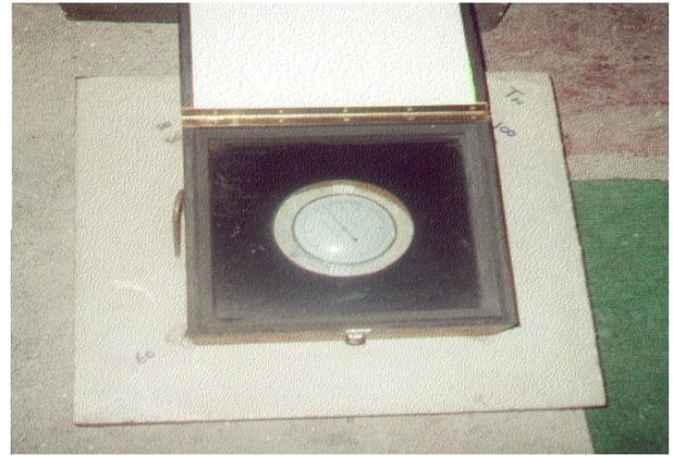
Figure 6: Surface Hygrometer test set-up.
