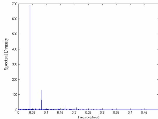
Figure 5 – Spectral periodogram for detached dwelling for metered profile over a six month period
