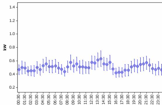
Figure 10 – Mean and 95% Confidence Intervals for detached dwelling over a six month period – synthetic profile
