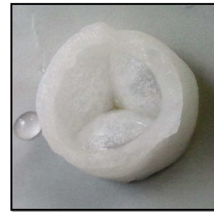
Figure 6. This image shows a sample of the 3-D CG material, post crosslinking and post infiltration with fibrin. The material stands up under its own weight and is easy to handle.
