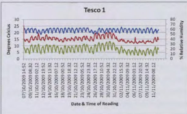
Fig. 7: During the cold October/November 2009 period, the main sales floor area was kept at a constant 20-23°C with the RH rarely going over 50%
